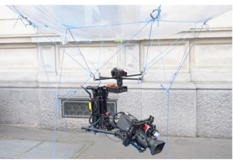
Max. operating wind speed: ~8,3 ms. (30 km/h.)
